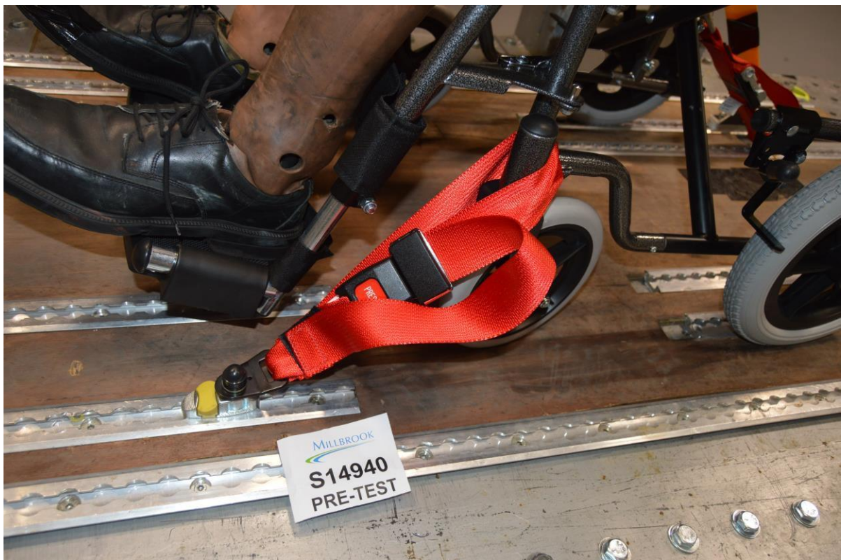
LH front tie-down, pre-test
