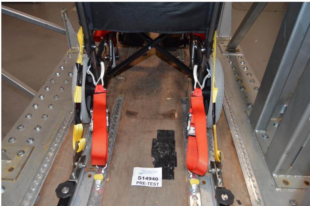
Rear tie-downs, pre-test
