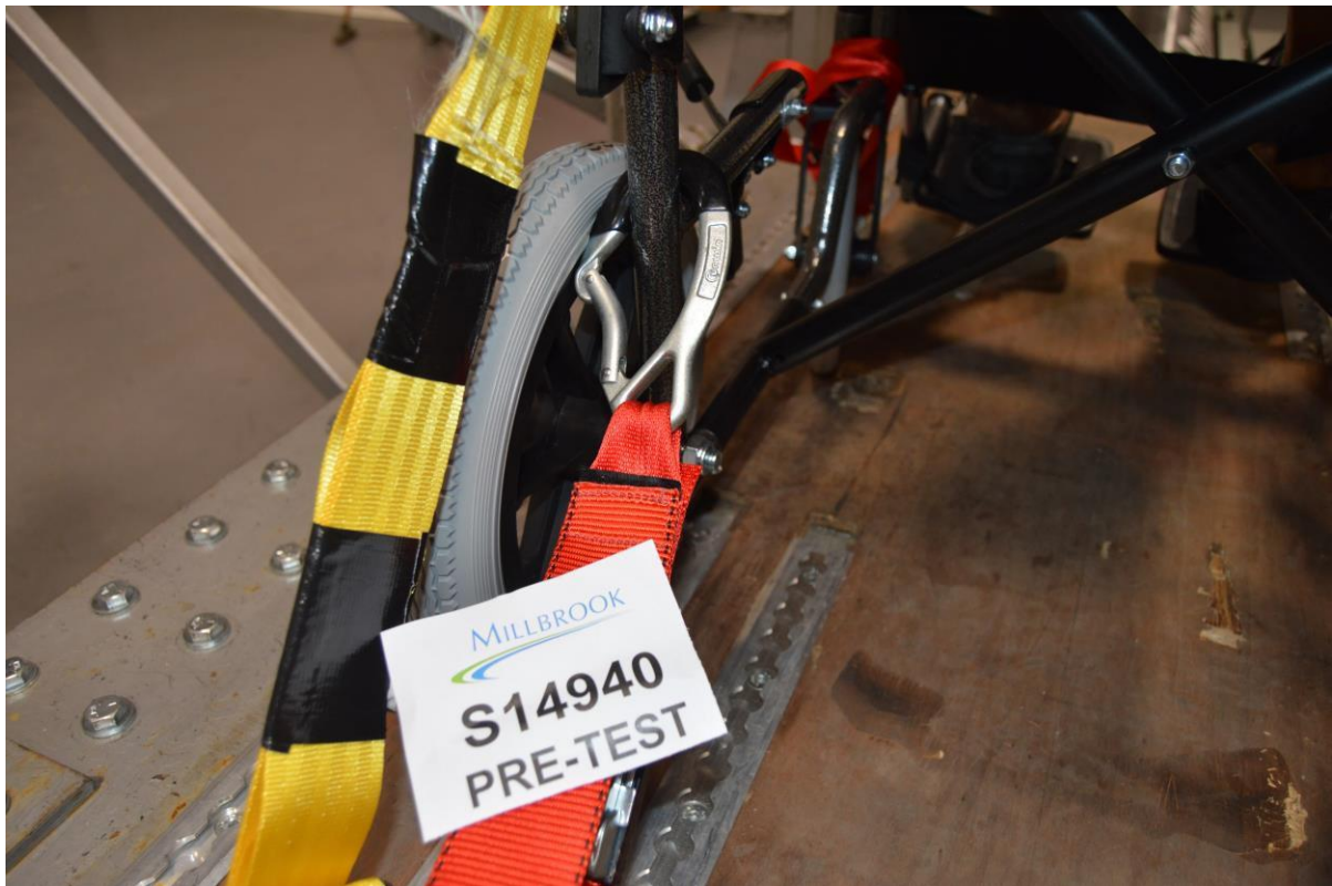
LH rear tie-downs, pre-test
