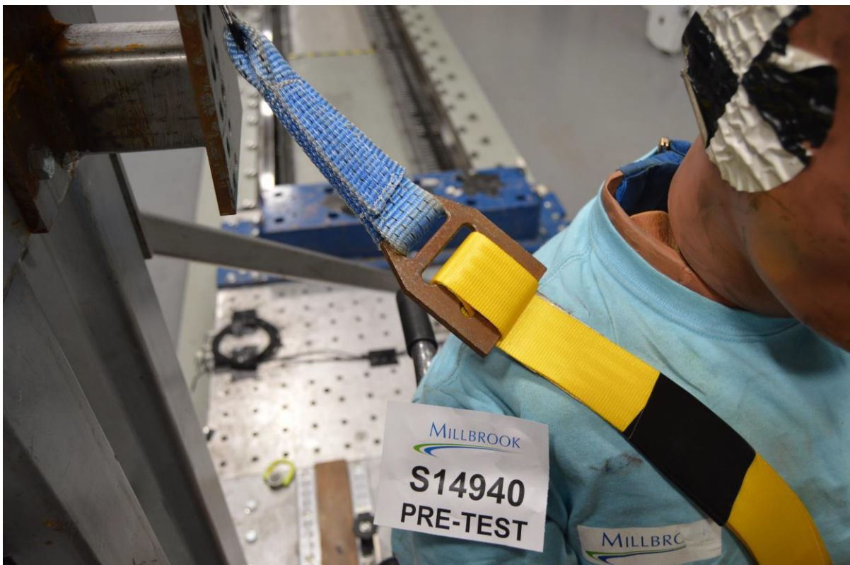
Upper torso restraint anchorage, pre-test
